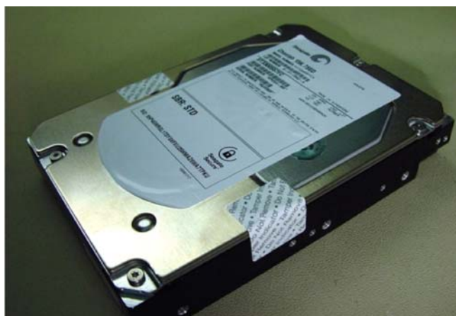
Figure 19. Example of FIPS tamper evidence labels.
